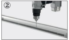
Using the pre-drilled gear rack as a guide, drill mounting holes in the track. Screw the gear rack to the track.
