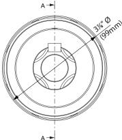
USE: Adapter for connecting Integrator carriages with motor.
