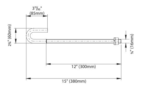
USE: Threaded anchor bolt for self-supporting carriages.
