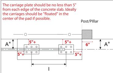
**Note:** The pad can start under the fence line. This is done to keep the gate face at no more than 2-1/4" from the fence line and to avoid entrapment.
