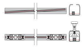
Position the first piece of gear rack inside the track. Use two template guides, one positioned at each end of the gear rack to center the gear rack lengthways within the track.
