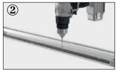
Using the pre-drilled gear rack as a guide, drill mounting holes in the track. Screw the gear rack to the track.
