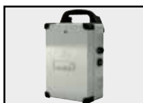
D113731 - ECOSOL BOX Interface for running BFT control panels off 24V solar power. Includes two 12V 7.2Ah batteries and circuit board for management of commands to control panel and battery charge management, with built-in Rolling Code 433.92 MHz receiver with 63 stored positions. Features carry handle for possible quick-charging of batteries from electrical power outlet through ECOSOL CHARGER accessory.
