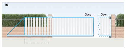
10 - Run the gate manually until it rests completely against the lower end cup situated on the pillar.
