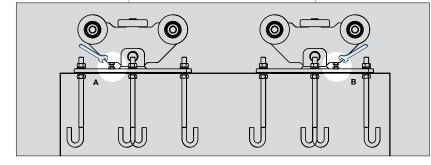
If the gates needs further adjustment, use the adjustment screws on the CGA models (as shown to left) and the bolts under the carriage/foundation plate on the steel models.
